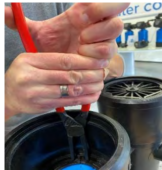
Fig. 14 circlip pliers for removal
