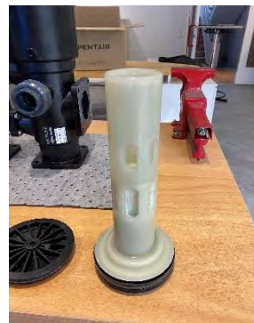
Fig. 12 Piston with O-ring
